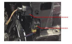
Disconnect the horn connectors on both sides of the vehicle.
