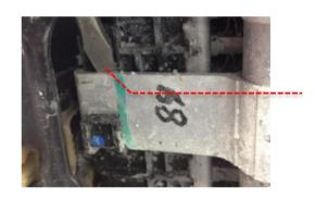
Disconnect the intercooler from the shroud by pressing the tabs on the yellow hanger clips, shown, while simultaneously lightly tapping the face of the clip with a small ball peen hammer. Disconnect both clips, lean the radiator/intercooler towards the engine and remove the yellow hanger brackets. Note the orientation of the clips for reinstallation. Place outside of the work area.
