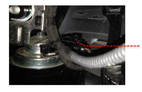
Disconnect the air temperature sensor located underneath the crash bar. Unclip the ambient sensor harness to disconnect the wiring from the radiator shroud.
