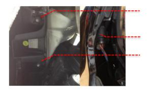
Disconnect the headlight harness on both headlights and remove the clip on the headlight wiring harness.
