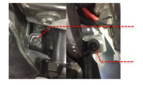
19 Remove the 2 x nuts from the crash bar studs.
